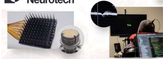
64-96 intracortical rigid elec/array (up to 6 arrays so far), tethered
