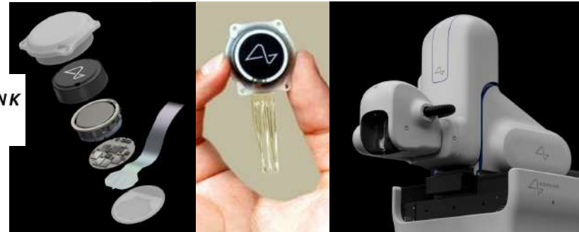
1024 intracortical flex elec/array, robot implantation, wireless
